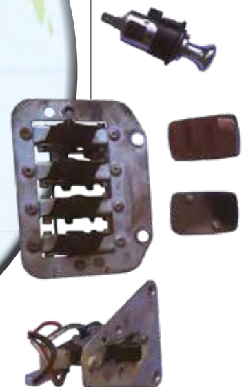
Door handle plates, electric window components and a replacement cigar lighter for the front seats were among the parts needed for the St Helena LWB Silver Shadow
