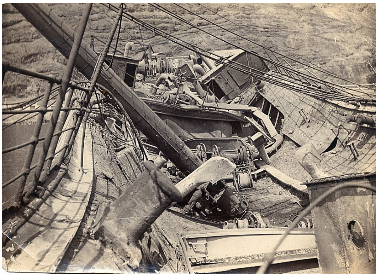
Fire-warped damage to the Papanui 19
