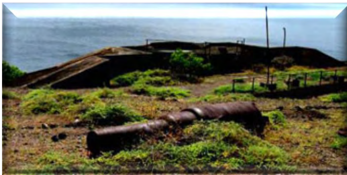
Upper Munden's Guns. Type: Armstrong Rifled Muzzle Loader (RML) with calibre of nine inches and weighing over 12 tons. Date: 1880s Range: three miles.
