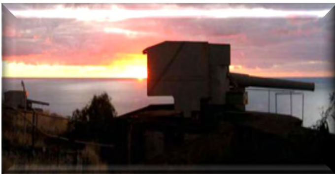
Ladder Hill Guns: Type: Elswick Mark VII wire breech loaders with a six inch calibre. Dated 1903. Maximum range with full charge and 30° elevation 25,000 yards. Standard naval and coastal defence guns for 50 years.
